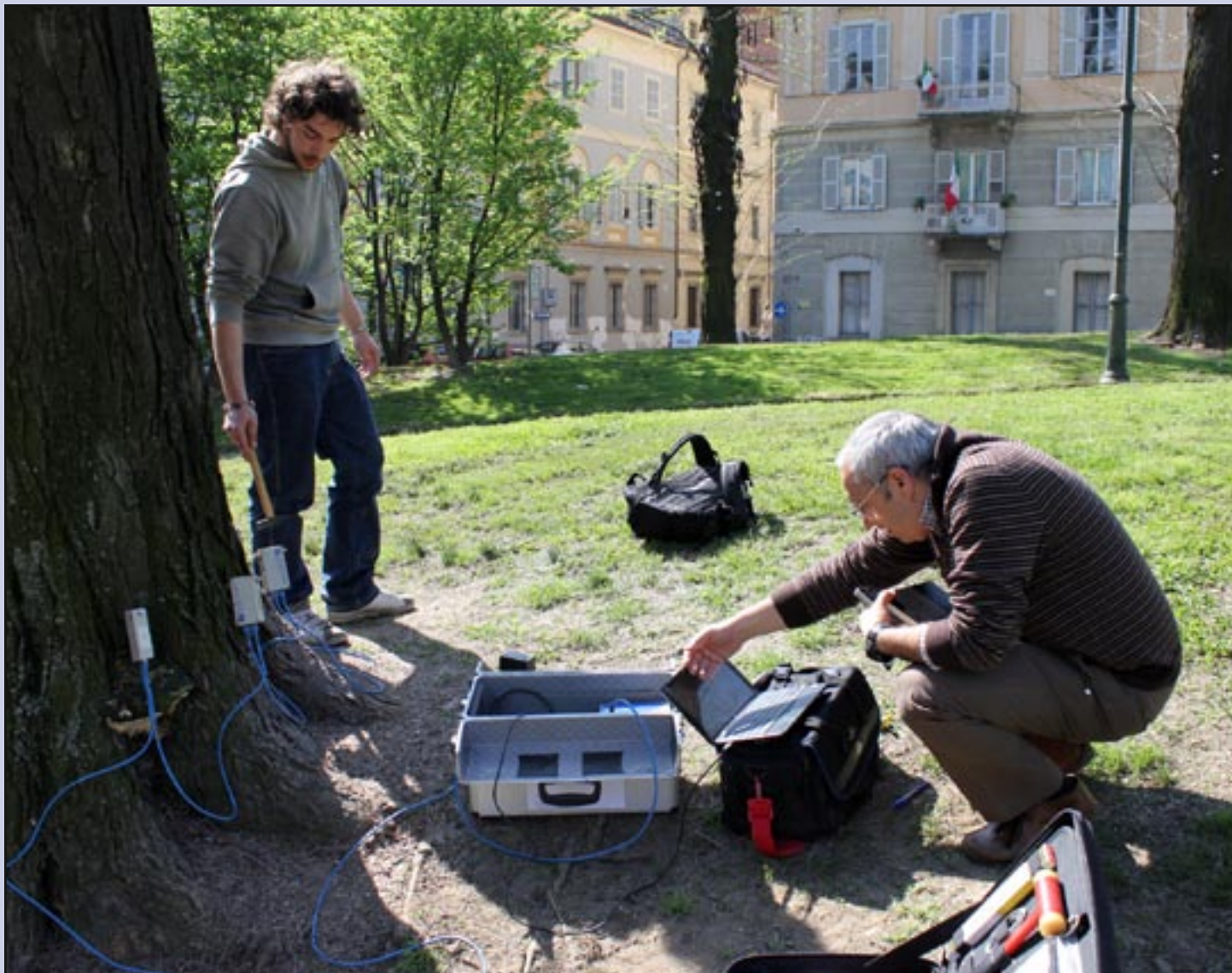
Structural diagnostics testing using sonic tomography
